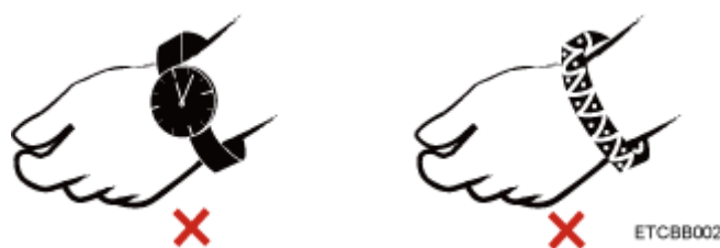
Figure 8-2 Removing conductive objects
