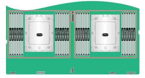
**Table 5-7** DDR5 memory modules installation guidelines (positions of the memory modules)
